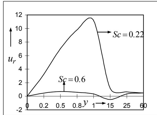
Figure 4: Velocity  $u_r$  against  $y$ , for variation of Schmidt number  $Sc$  when  $Du=0.5$ ,  $Sr=2$ ,  $Pr=0.71$ ,  $Re=0.5$ ,  $\varepsilon=0.001$ ,  $Gr=10$ ,  $Gm=5$ ,  $\omega=0.5$ ,  $t=1$ ,  $U=0.5$  and  $z=0.25$ .
