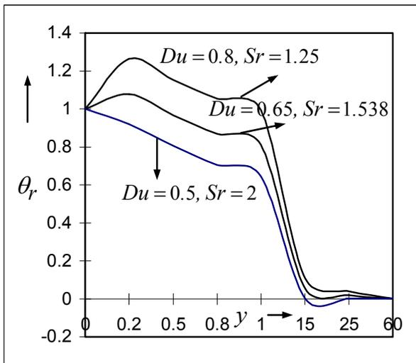
Figure 2: Temperature  $\theta_r$  against  $y$ , for variations of Dufour and Soret numbers  $Du$  and  $Sr$  respectively, when  $Sc=0.22$ ,  $Pr=0.71$ ,  $Re=0.5$ ,  $\varepsilon=0.001$ ,  $Gr=10$ ,  $Gm=5$ ,  $\omega=0.5$ ,  $t=1$ ,  $U=0.5$  and  $z=0.25$ .
