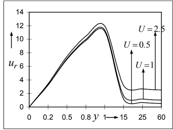
Figure 9: Velocity  $u_r$  against  $y$ , for variation of  $U$  when  $Du=0.5$ ,  $Sr=2$ ,  $Pr=0.71$ ,  $Re=0.5$ ,  $\varepsilon=0.001$ ,  $Gm=5$ ,  $Sc=0.22$ ,  $\omega=0.5$ ,  $t=1$ ,  $Gr=10$  and  $z=0.25$ .
