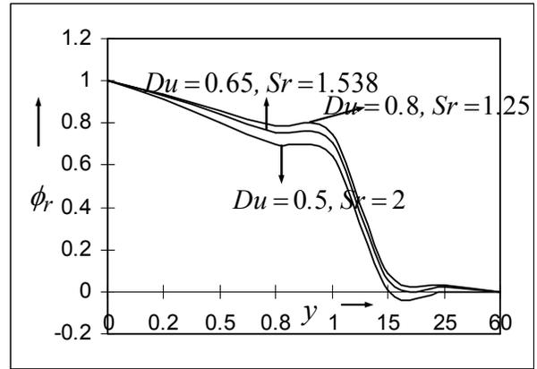
Figure 3: Concentration  $\phi_r$  against  $y$ , for variations of Dufour and Soret numbers  $Du$  and  $Sr$  respectively, when  $Sc=0.22$ ,  $Pr=0.71$ ,  $Re=0.5$ ,  $\varepsilon=0.001$ ,  $Gr=10$ ,  $Gm=5$ ,  $\omega=0.5$ ,  $t=1$ ,  $U=0.5$  and  $z=0.25$ .
