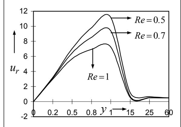
Figure 10: Velocity  $u_r$  against  $y$ , for variation of suction Reynolds number  $Re$  when  $Du=0.5$ ,  $Sr=2$ ,  $Pr=0.71$ ,  $U=0.5$ ,  $\varepsilon=0.001$ ,  $Gm=5$ ,  $Sc=0.22$ ,  $\omega=0.5$ ,  $t=1$ ,  $Gr=10$  and  $z=0.25$ .
