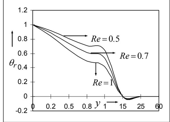
Figure 11: Temperature  $\theta_r$  against  $y$ , for variation of suction Reynolds number  $Re$  when  $Du=0.5$ ,  $Sr=2$ ,  $Pr=0.71$ ,  $Sc=0.22$ ,  $\varepsilon=0.001$ ,  $Gr=10$ ,  $Gm=5$ ,  $\omega=0.5$ ,  $t=1$ ,  $U=0.5$  and  $z=0.25$ .
