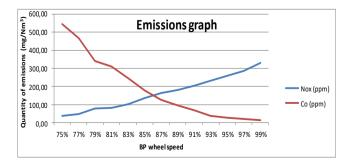
Figure 8. Turbine emissions curve
