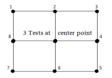
Figure 2. Experimental points of the two-factor centered-face composite plane
