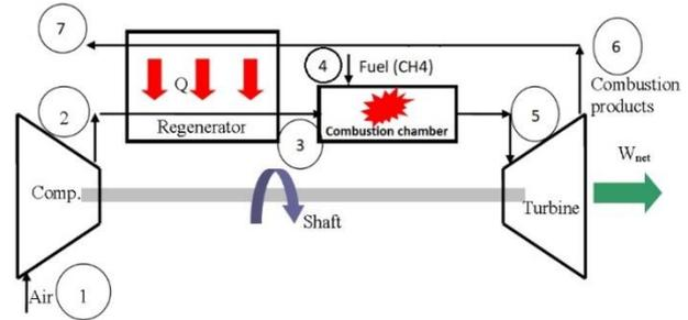
**Figure 2.** Regenerative gas turbine power plant
