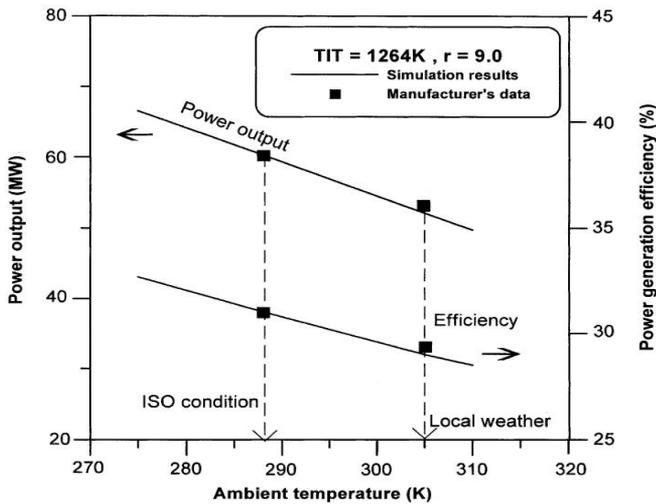
**Figure 1.** Effect of entry temperature on the power output and power generation efficiency of the GT [2]
