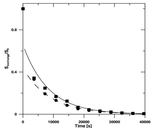
**Figure 10.** Reduction of the exchange surface during the drying process (■ form (1), ● form (2))
