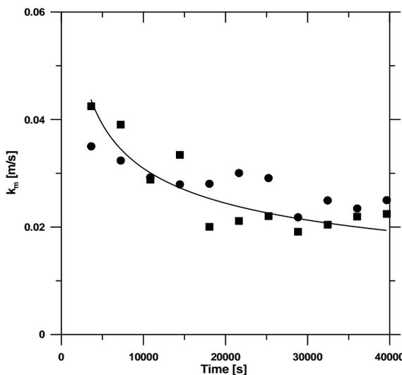
**Figure 7.** Convective mass transfer coefficient during the drying process (■ form (1), ● form (2))
