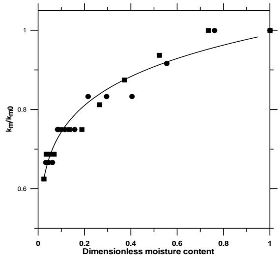
**Figure 8.** Evolution of the convective mass transfer with the moisture content (■ form (1), ● form (2))
