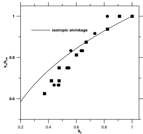
**Figure 9.** Evolution of the convective mass transfer with the shrinkage ratio (isotropic shrinkage:  $k_m/k_{m0} = S_b^{1/3}$ ) (■ form (1), ● form (2))
