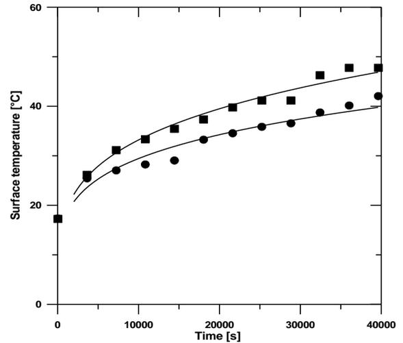
Figure 4. Measured surface temperature during the drying process (■ form (1), ● form (2))
