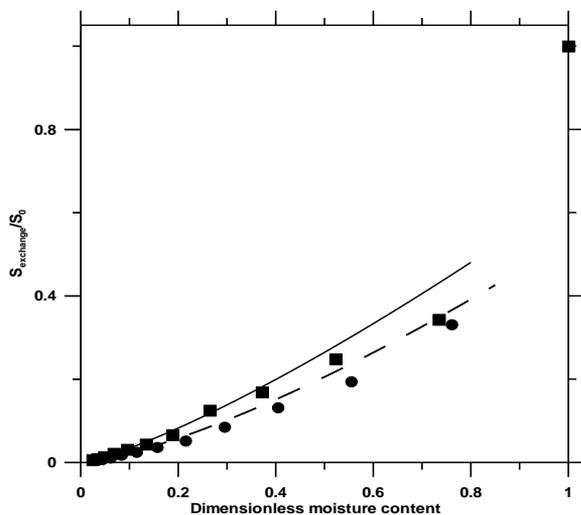
**Figure 11.** Reduction of the exchange surface with moisture content (■ form (1), ● form (2))
