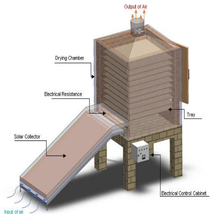
Figure 1. Experimental solar dryer
