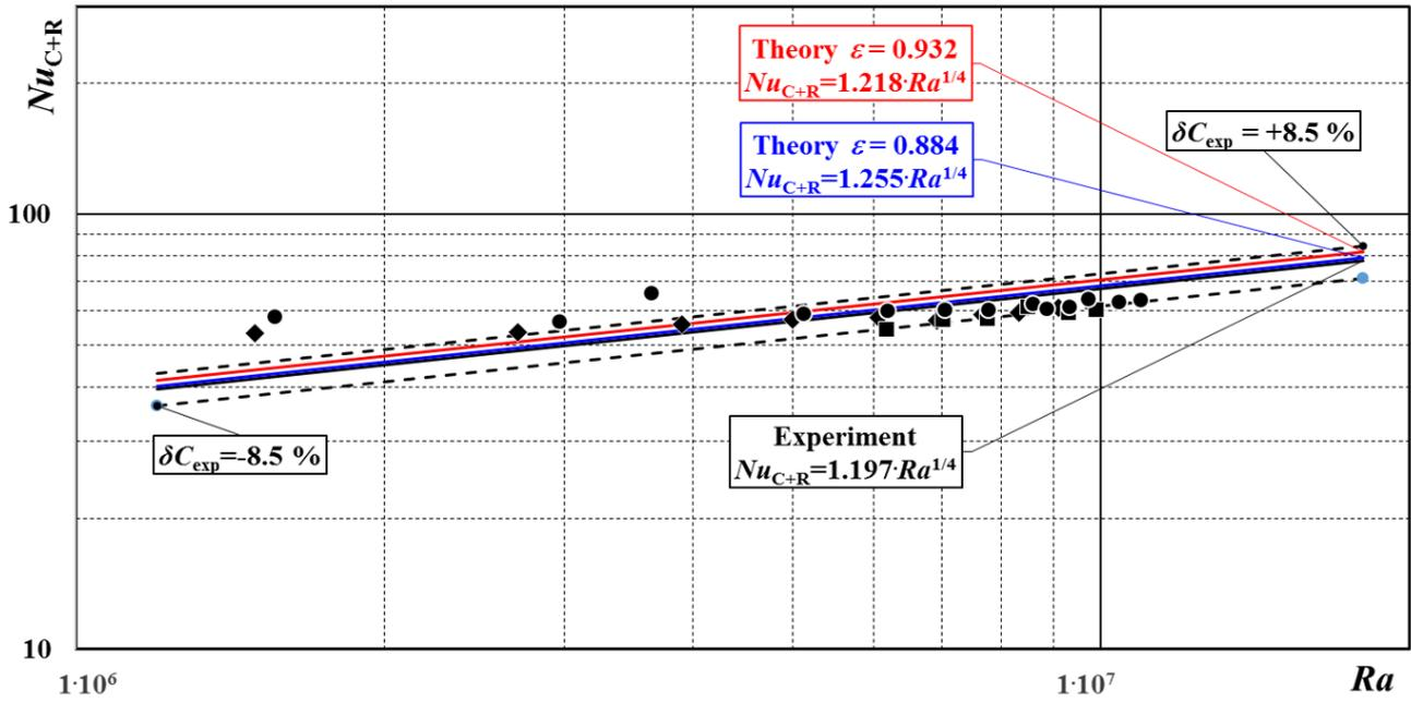
**Figure 8.** The results of the experimental tests, some of which - from Series I (diamonds) and Series II (squares) - are included in Table 3, and the remaining (Series III) experimental points (shown by dots) are not shown in Table 3. The black line shows the approximation of all the experimental results (41). The theoretical solution obtained for  $\varepsilon=0.884$  is shown by the blue line, and the one for  $\varepsilon=0.932$  by the red line
