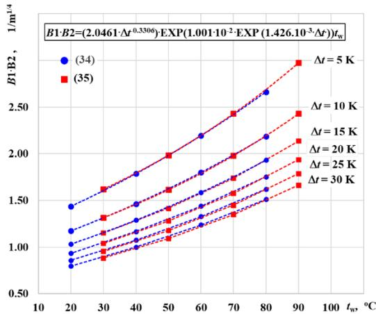
**Figure 4.** Comparison of values of  $B1 \cdot B2$  calculated from Eqns. (34) (blue circles) and (35) (red squares). Eq. (36), shown in the box, is the result of the approximation of the curves obtained using Eq. (34)
