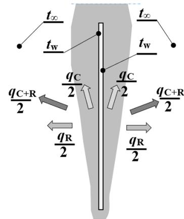
**Figure 2.** Draft scheme of a thin, double-sided, heated isothermal vertical plate
