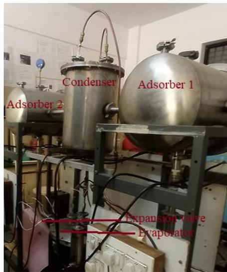
Figure 7. Picture of the two bed adsorption refrigeration test setup
