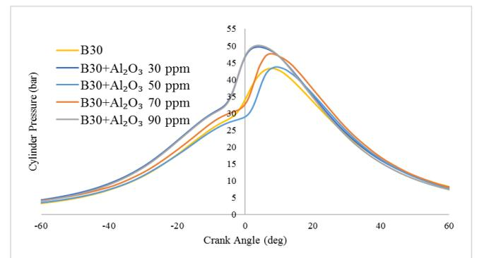
Figure 9. Cylinder pressure at crank angle
