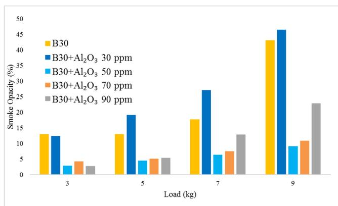
Figure 11. Smoke opacity at different engine loads
