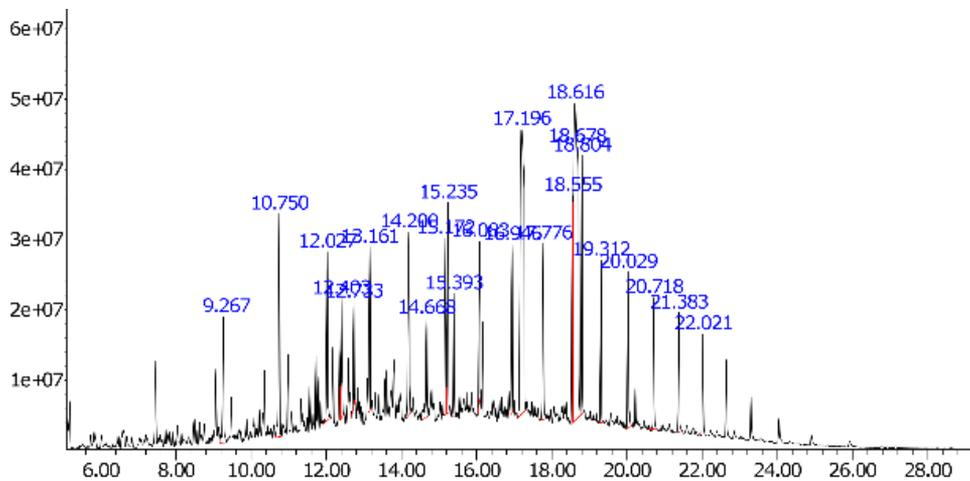
Figure 4. GC-MS Biodiesel B30
