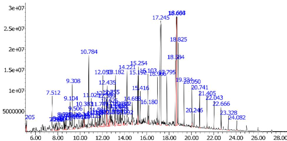
Figure 6. GC-MS B30+Al<sub>2</sub>O<sub>3</sub> nanoparticle
