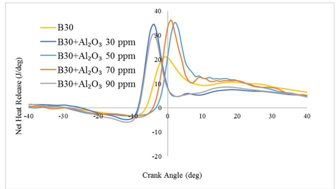
Figure 8. Net heat release at crank angle
