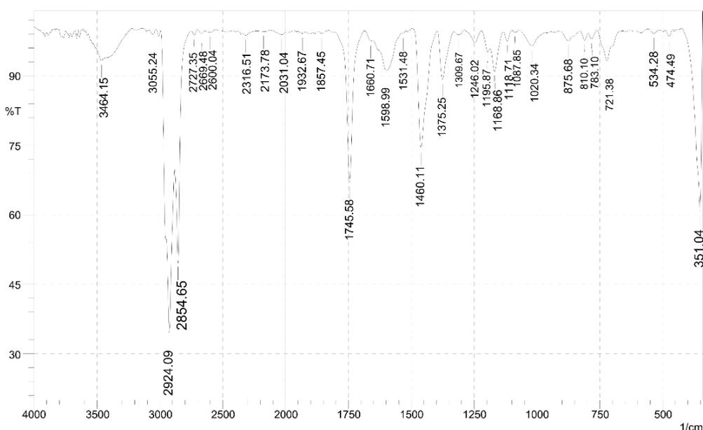
**Figure 3.** FTIR biodiesel B30
