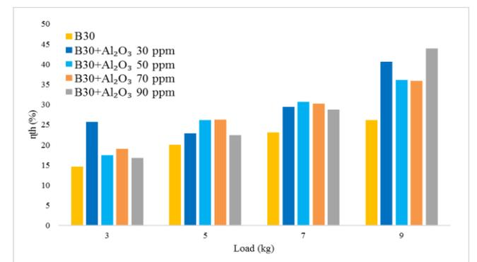
Figure 10. Brake thermal efficiency at different engine loads
