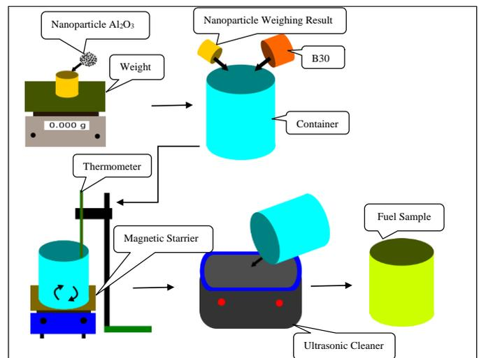
Figure 2. Preparation of biodiesel with nanoparticle  $Al_2O_3$
