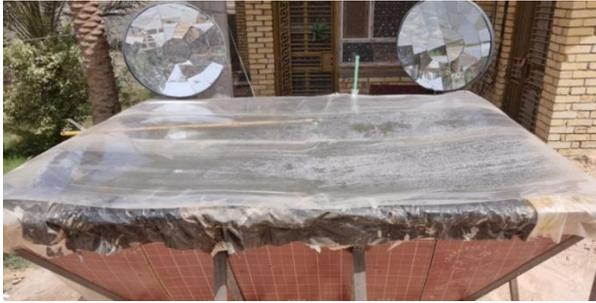
Figure 2. Solar pond with plastic cover and reflective mirrors
