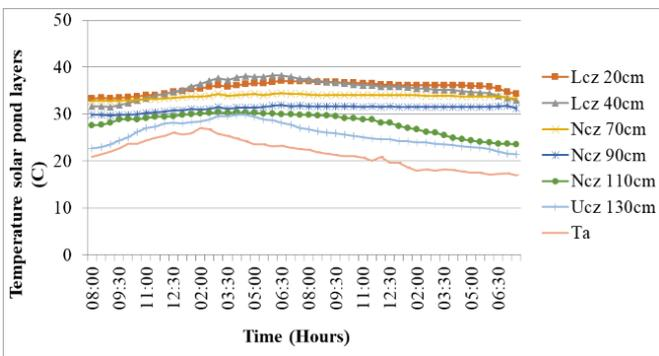
Figure 5. Three-layer salinity solar pond's temperatures
