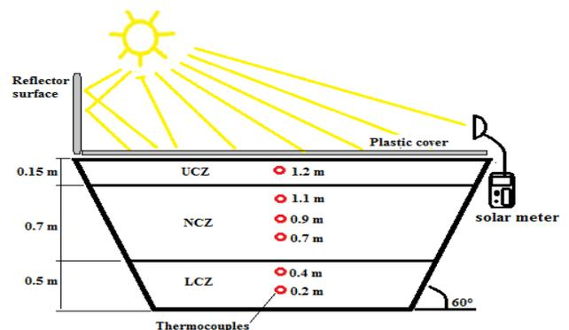
Figure 1. Schematic of the solar pond
