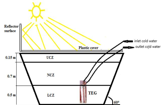
Figure 4. The location of the TEG fixation inside the pond
