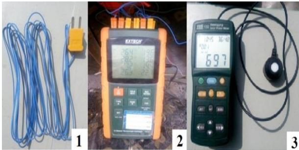
Figure 3. Instruments for measuring: 1-thermocouples, 2-temperature meter, 3-solar power meter
