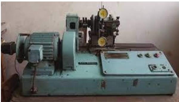
**Figure 3.** Combined bending - Torsion fatigue testing machine
