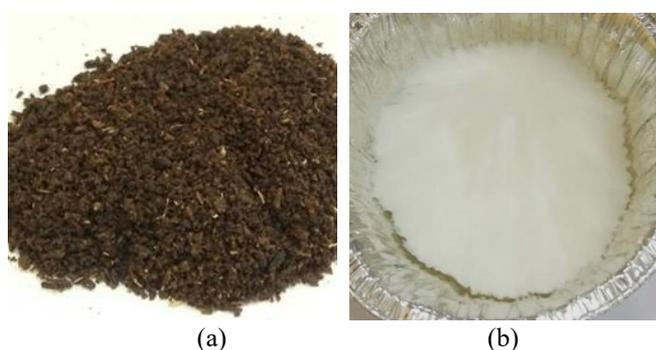
**Figure 1.** (a) Dried banana peel and (b) CCNF-40 product
