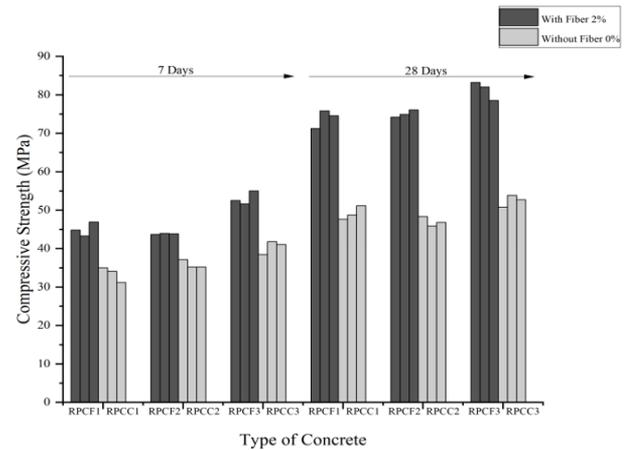
**Figure 6.** Effect of varying the river sand (RS) content on the compressive strength of RPCF, at 7 and 28 days
