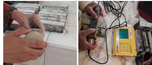
**Figure 2.** Ultrasonic device
