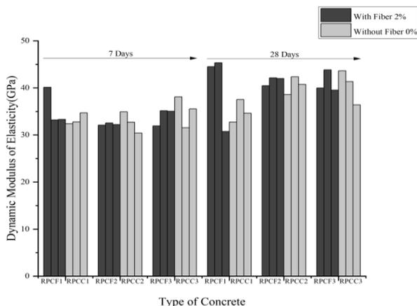
**Figure 8.** Effect of sand percentage variation on the dynamic modulus of elasticity of RCPFs, at 7 and 28 days
