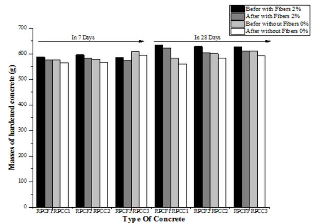
**Figure 4.** Histogram representing the masses of prismatic specimens before and after storage in water, at 7 and 28 days
