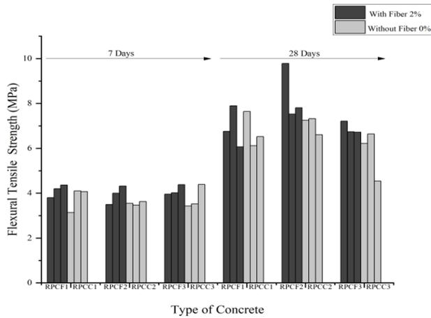
**Figure 7.** Effect of sand percentage variation on the flexural tensile strength of RCPFs, at 7 and 28 days
