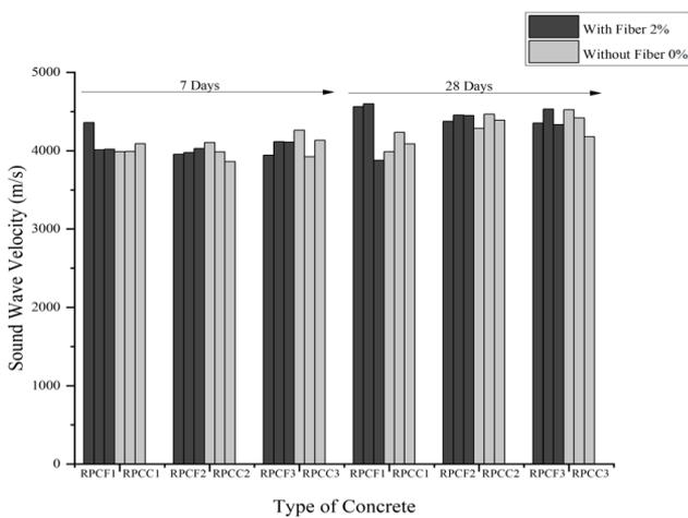
**Figure 5.** Evolution of the sound wave velocity of the different RPCFs at 7 and 28 days
