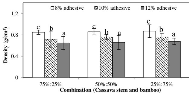
**Figure 3.** Effect of briquette combination and adhesive concentration on the density of charcoal briquettes (different letters within a combination show significant different at a 5% significance level between adhesive content using Duncan's multiple-range tests)
