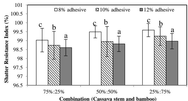
**Figure 5.** Effect of briquette combination and adhesive concentration on shatter resistance index of charcoal briquettes (different letters within a combination show significant different at a 5% significance level between adhesive content using Duncan's multiple-range tests)
