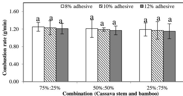
**Figure 6.** Effect of briquette combination and adhesive concentration on combustion rate of charcoal briquettes (different letters within a combination show significant different at a 5% significance level between adhesive content using Duncan's multiple-range tests)
