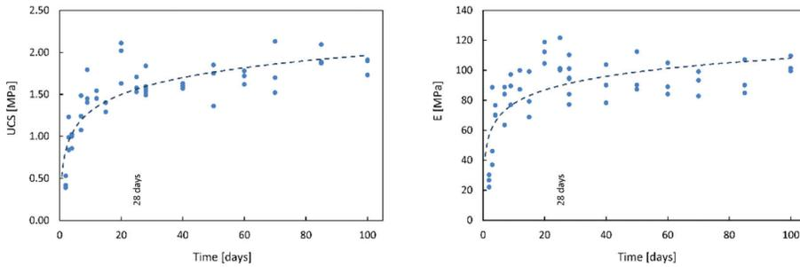
Figure 3: Evolution of UCS (left) and elastic modulus (right) for L12 specimens.
