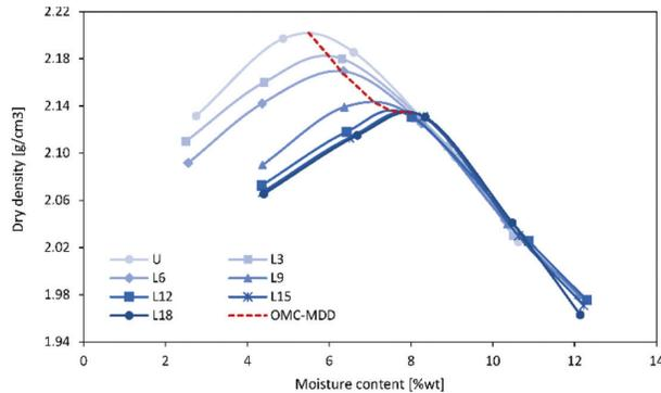
Figure 1: Dry density as a function of the moisture content for the RE mixtures according to Modified Proctor test.
