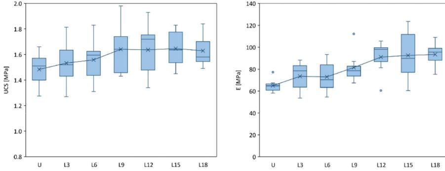
Figure 2: UCS (left) and elastic modulus (right) of RE specimens at 28 days.
