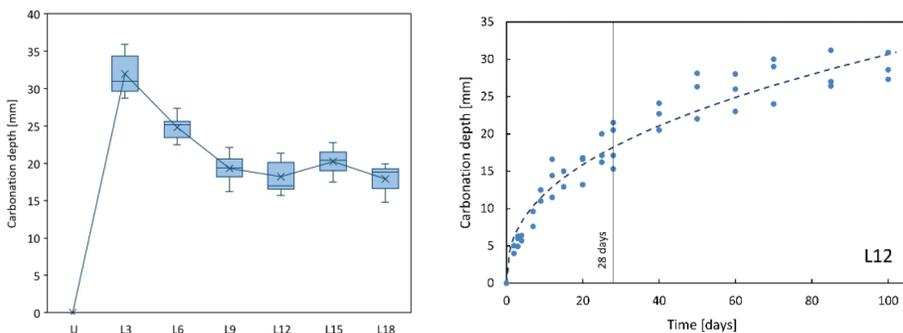
Figure 4: Carbonation depth for different RE mixtures at 28 days (left) and evolution of carbonation during curing time for L12 specimens (right).
