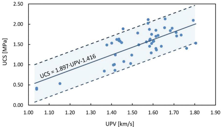
Figure 5: UCS as a function of the ultrasonic pulse velocity.
