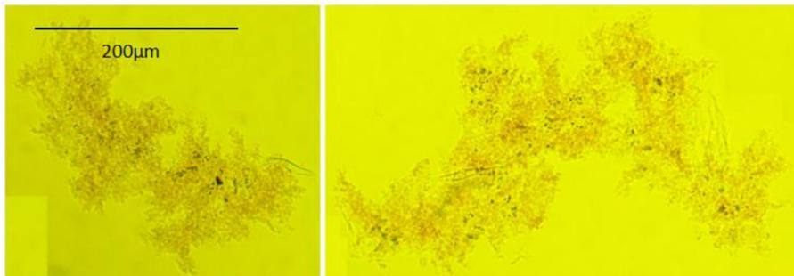
Figure 3: Particles formed by coagulation in still liquids.
