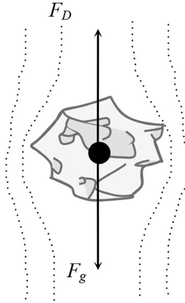
Figure 5: Forces acting on a spherical particle sediment in a fluid.
