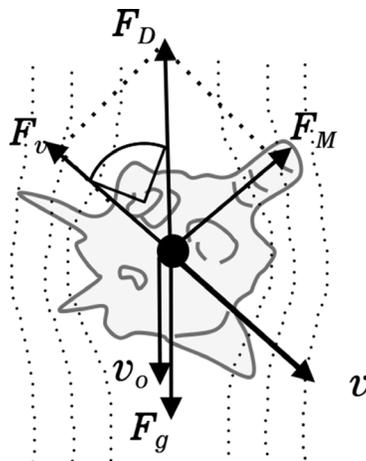
Figure 6: Forces acting on a non-spherical particle falling in a fluid.
