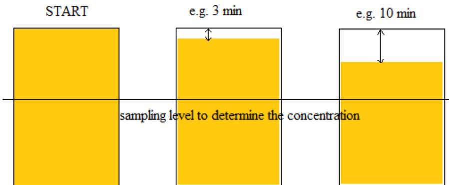
Figure 8: Determination of the sedimentation velocity of monodisperse suspensions in an experimental way.
