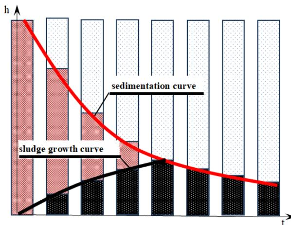
Figure 4: The sedimentation process of the monodisperse mixture.
