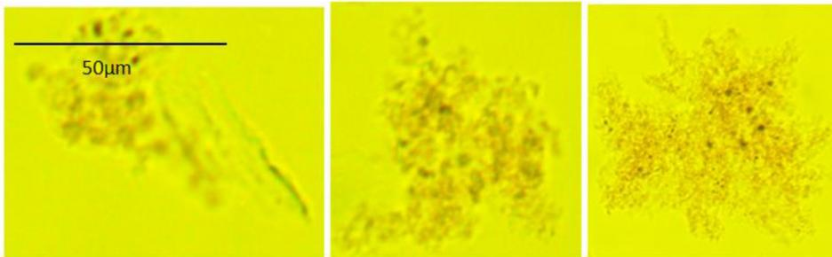
Figure 2: Particles formed by coagulation in flow devices.
