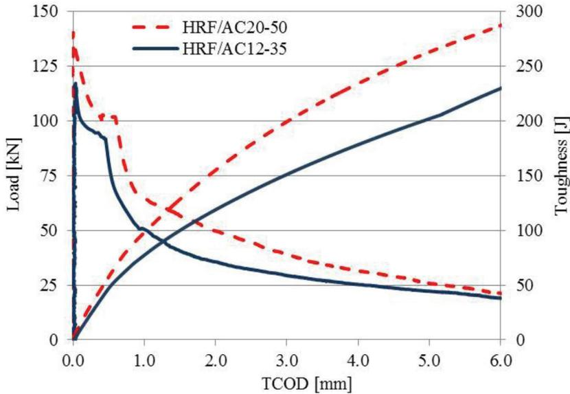
Figure 3: Curves of vertical load–total crack width obtained with the BCN test.
