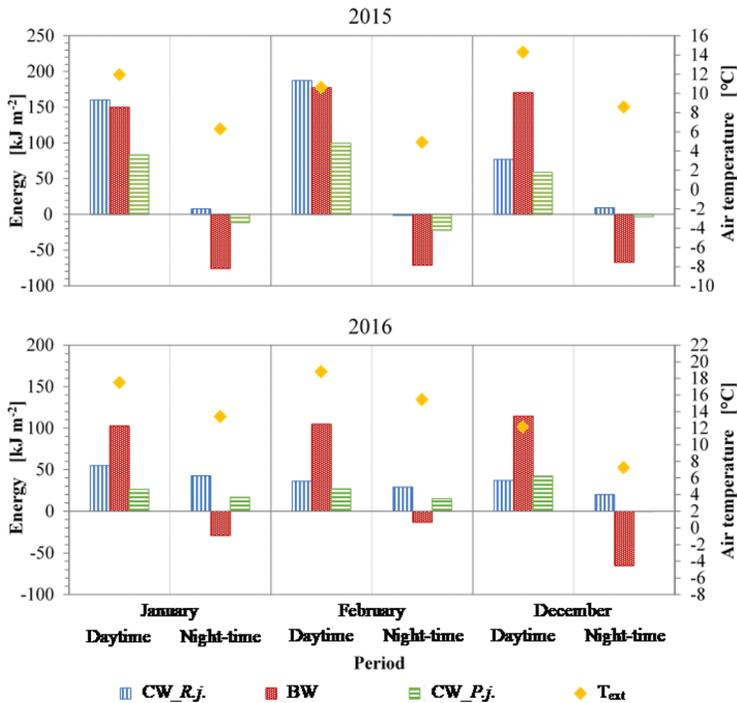
Figure 4: Overall cumulative energy transfer through the bare wall (BW) and the walls covered with *Rhynchospermum jasminoides* (CW\_R.j.) and *Pandorea jasminoides* (CW\_P.j.) (primary axis); average daytime and night-time external air temperature ( $T_{ext,a}$ ) (secondary axis).
