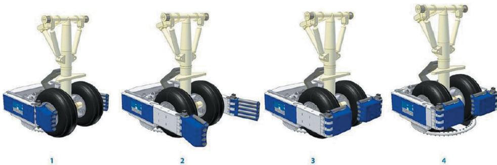
Figure 3: TaxiBot front wheel locking system (courtesy of IAI-TLD).
