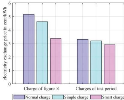
Figure 9: Cost of charges with the German electricity exchange price.
