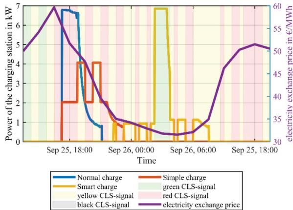
Figure 8: Simulation of the three charging modes and of the trend of German electricity exchange price.
