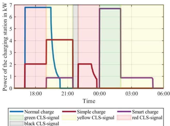
Figure 2: Charging mode Normal, Simple and Smart.
