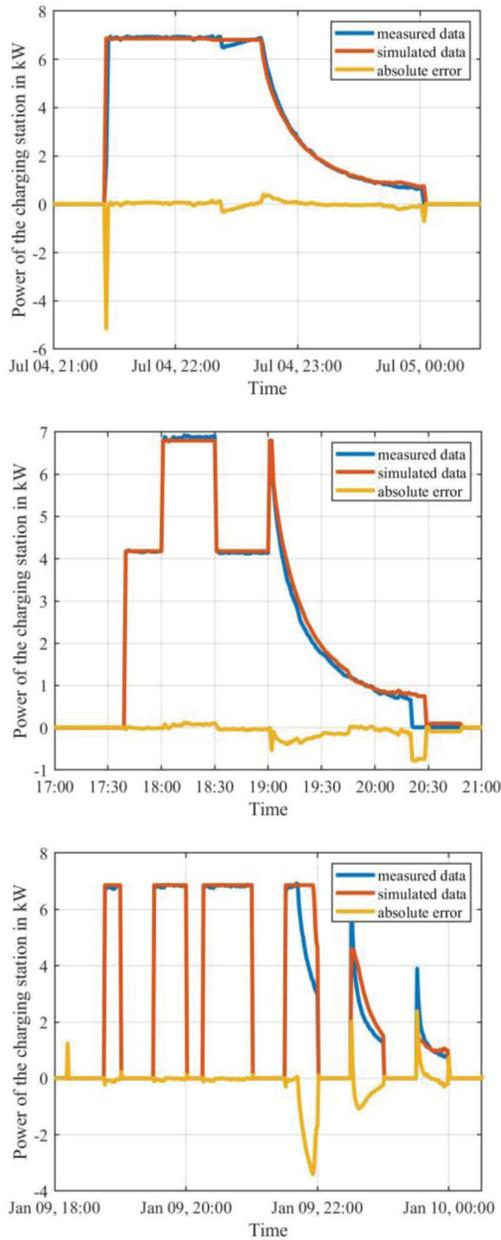
Figure 3: Measured data, simulated data and absolute error of the three charging modes.
