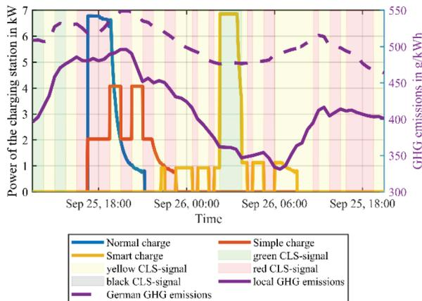
Figure 6: Simulation of the three charging modes and of the trend of the greenhouse gas emissions in the German and local electricity grid.
