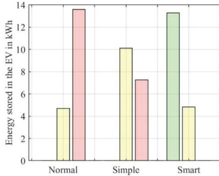
Figure 4: Load shifting of the three charging modes for the charge of Fig. 2.
