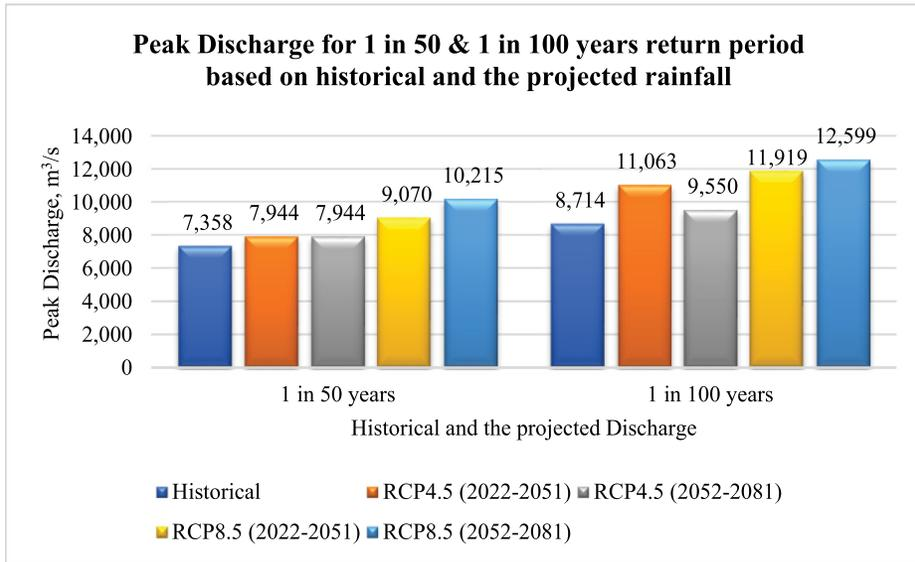
Figure 6: Peak discharge ( $\text{m}^3/\text{s}$ ) in 1 in 50 & 1 in 100 years return period based on historical and the projected future discharge.
