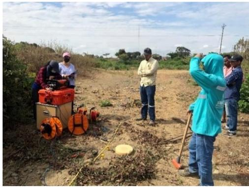
Figure 4. Field data collection of seismic line 1 (SR1)
