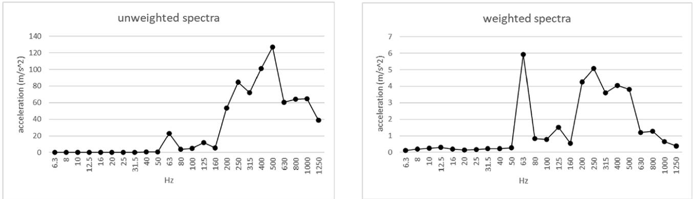
**Figure 4.** Unweighted and weighted spectra (three-axial acceleration x,y,z) of the hammer measured directly on the handle
