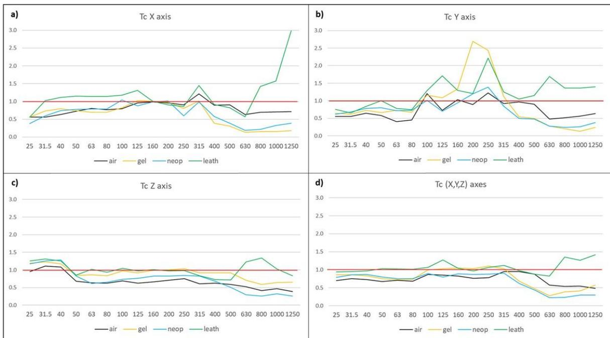
Figure 7. Total three-axes transmissibility and along each single axis
