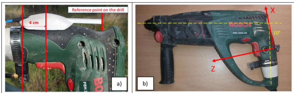
Figure 2. Position of the accelerometers
