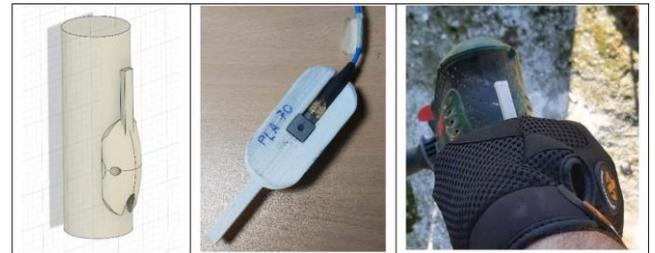
Figure 1. 3-D printed adaptor with longitudinal landmark
