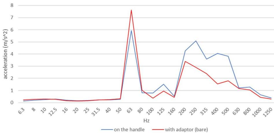
Figure 5.  $W_h$  triaxial acceleration measured directly on the handle of the hammer and with bare-hand adaptor
