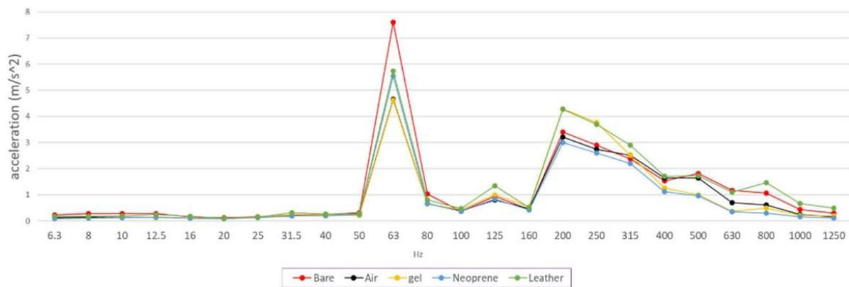
Figure 6.  $W_h$  three-axial accelerations measured on the bare-hand adaptor and wearing gloves
