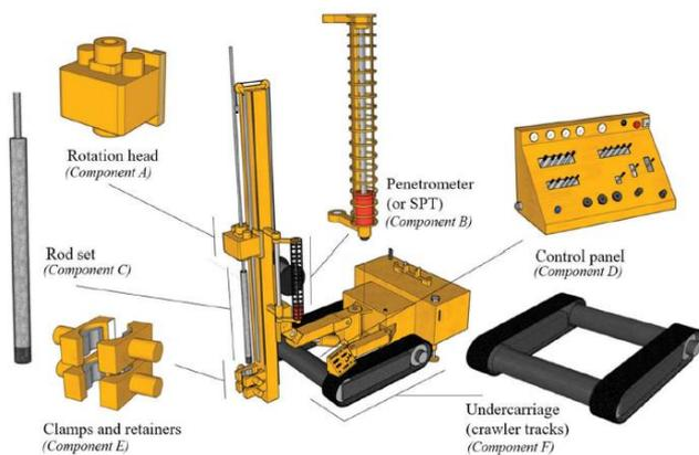
Figure 4. Drilling machine 3D model in Sketchup®
