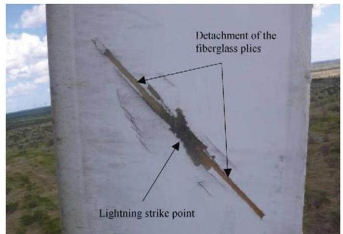
Figure 2. Damage from lightning to a turbine blade [10]
