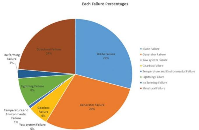
Figure 3. Wind turbine failure rates
