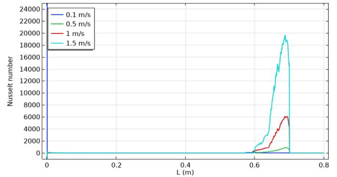
**Figure 18.** Nusselt number in channel-cavity assembly for different inlet air velocity
