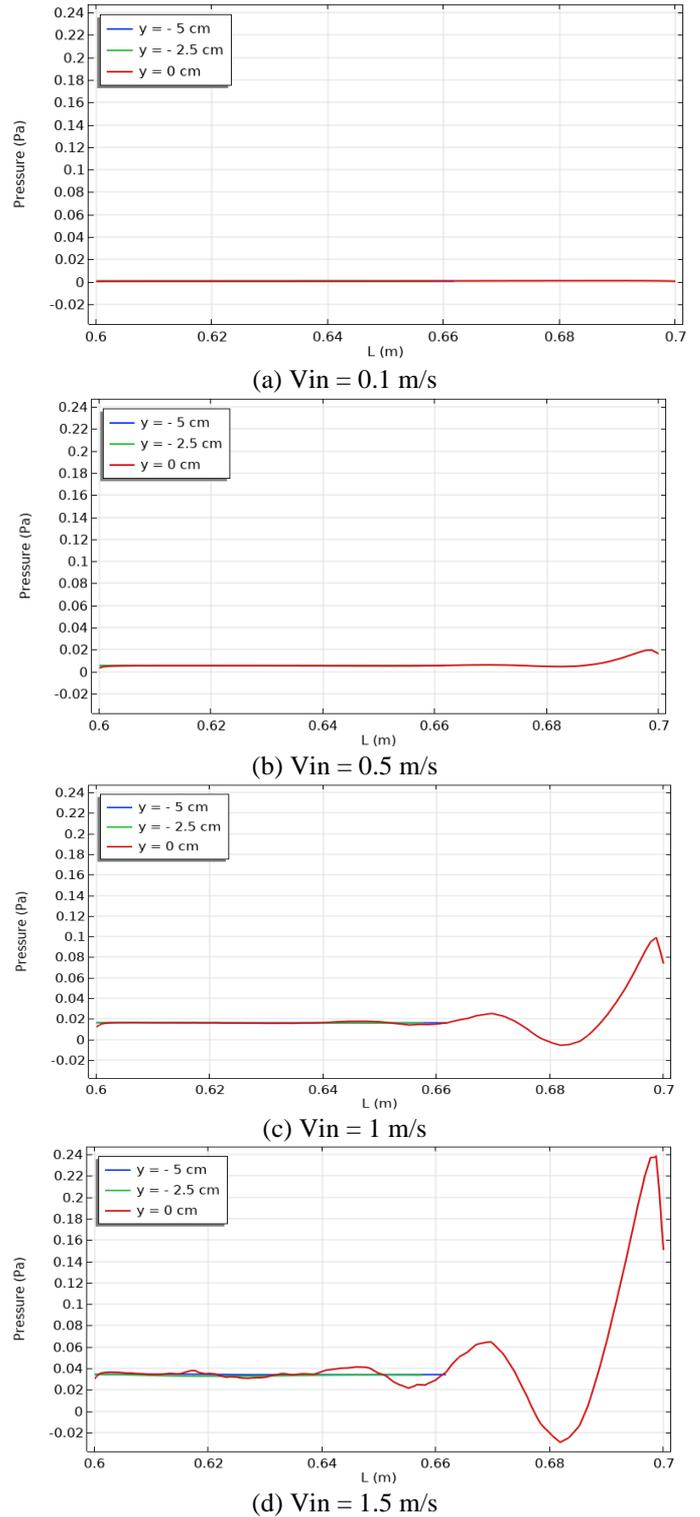
**Figure 12.** Pressure profile during negative y-axis in the cavity at a different inlet velocity
