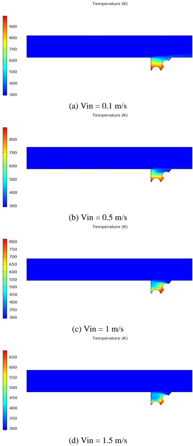
**Figure 5.** 2D passage temperature contours at a different inlet velocity
