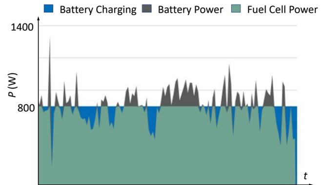
**Figure 3.** Power supply (fuel cell + battery) power trend
