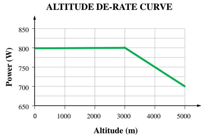
**Figure 4.** Fuel cell power reduction with altitude
