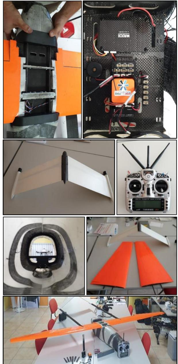
Figure 6. Components and prototype of the scale model
