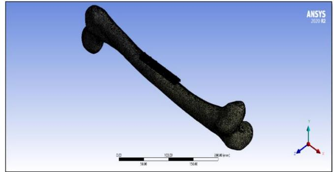
**Figure 3.** Meshed femur bone with plate fixation
