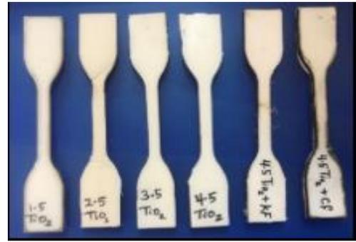
Figure 1. Biocomposites specimen for tensile test
