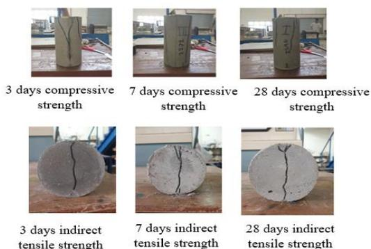
Figure 7. Mixed I crack pattern of lightweight concrete
