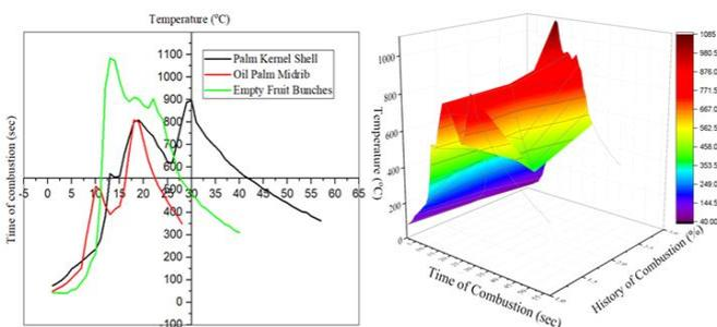
Figure 5. The combustion temperature effect of different fuels at the M-1 point
