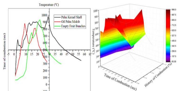
Figure 7. The combustion temperature effect of different fuels at the M-2 point
