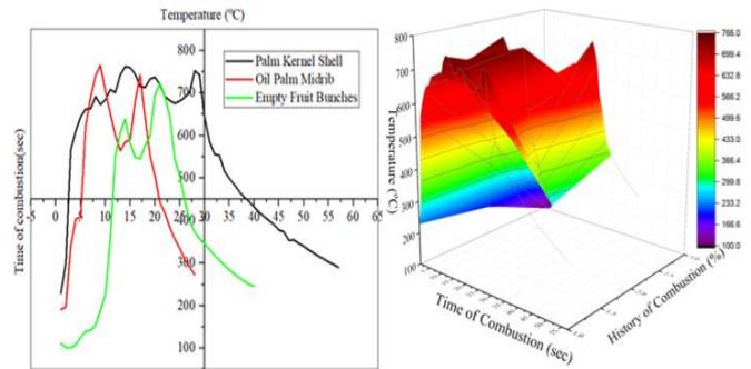
**Figure 11.** The combustion temperature effect of different fuels at the M-4 point
