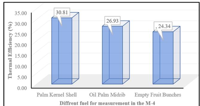
**Figure 12.** Thermal efficiency at M-4 points with different fuels
