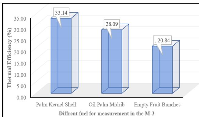
**Figure 10.** Thermal efficiency at M-3 points with different fuels
