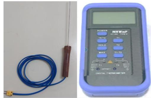
**Figure 3.** Digital thermometer merk HotTemp HT-306
