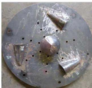
**Figure 2.** Modification of perforated plate with the addition of three spoons
