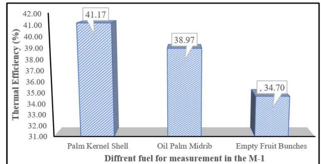
Figure 6. Thermal efficiency at M-1 points with different fuels
