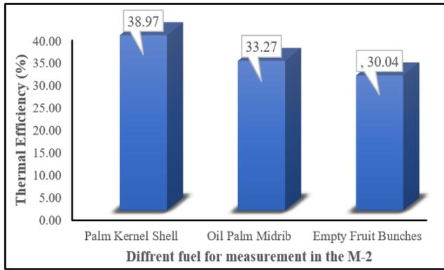
**Figure 8.** Thermal efficiency at M-2 points with different fuels
