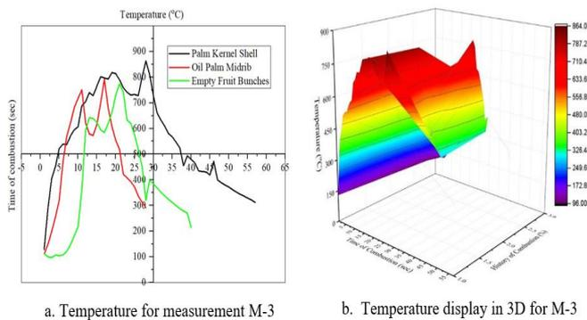
**Figure 9.** The combustion temperature effect of different fuels at the M-3 point
