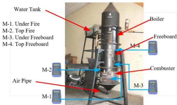
**Figure 1.** Schematic diagram for fluidized-bed combustor (FBC)
