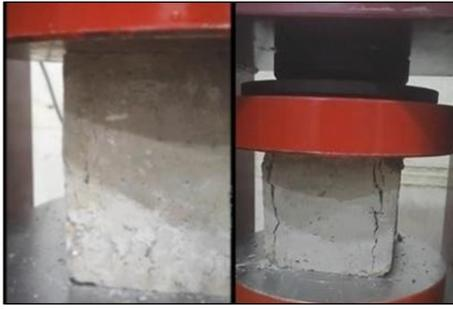
**Figure 6.** Compression test results for traditional concrete and concrete with SFRC
