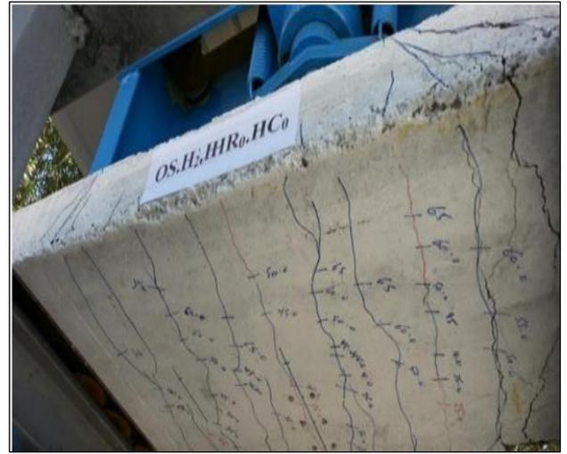
Figure 4. Mode of failure and cracks pattern of HCS [3]
