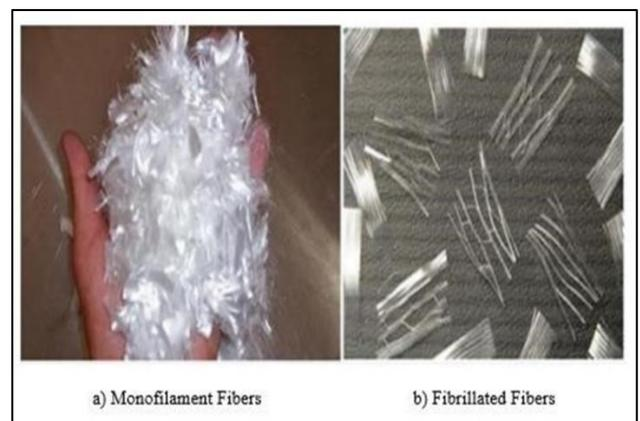
Figure 3. Polypropylene Fibers [17]
