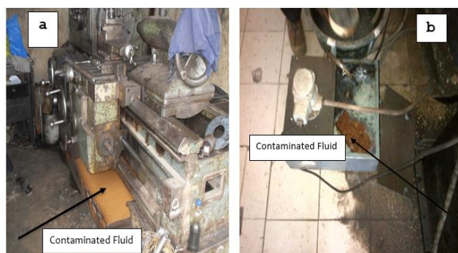
Figure 6. (a) Exposed machine sump with three weeks emulsion cutting fluid (b) Exposed machine sump with five months emulsion cutting fluid
