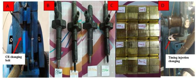
Figure 10. Selected design parameters A-VCR B-IP changing C-M range D-TI setting
