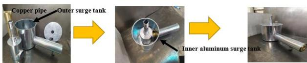
Figure 2. Diesel engine cooler EGR system parts
