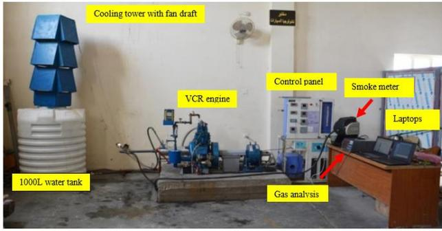
Figure 6. Front view of the experimental set up
