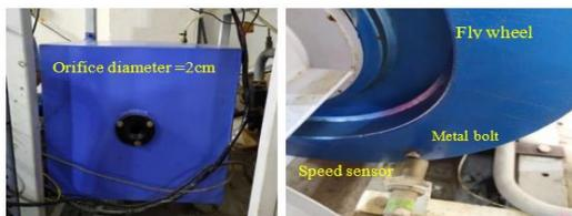
Figure 8. (left) air box and (right) engine speed sensor setup
