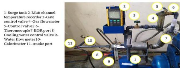
Figure 3. Diesel engine cooler EGR system setup
