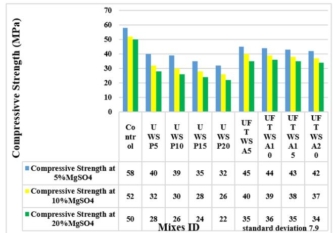
**Figure 12.** Influence of MgSO<sub>4</sub> Solution on Compressive Strength of Mortar
