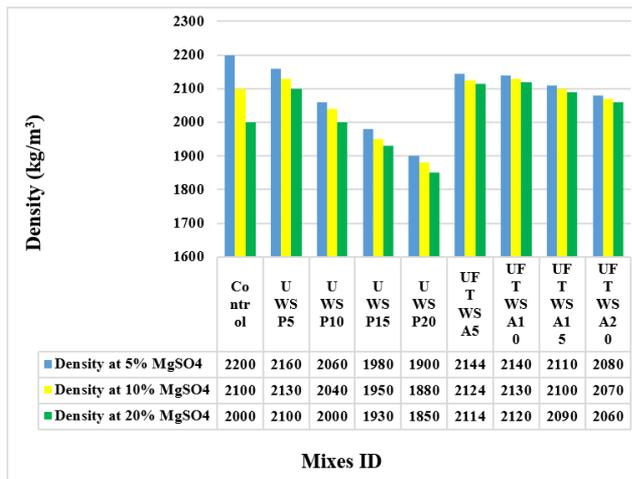
**Figure 11.** Influence of MgSO<sub>4</sub> Solution on Dry Density of Mortar
