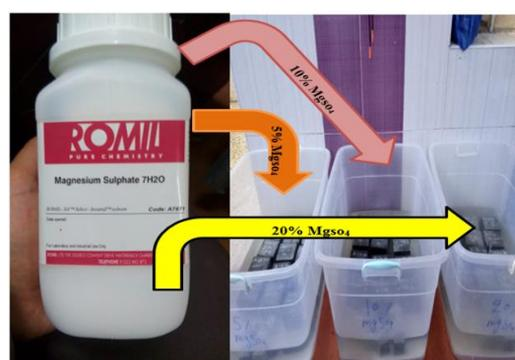
**Figure 4.** Curing mortar specimen in magnesium sulfate acid (MgSO<sub>4</sub>) solution
