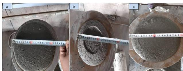
**Figure 3.** Slump flow test (a) control mix (b) M-5% UWSP (c) M-5% UFTWSA
