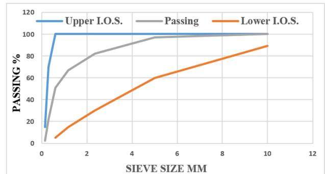
Figure 1. Grading curve for Fine aggregate
