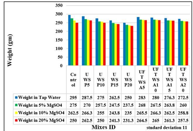
**Figure 14.** Weight of the Specimens for Control, UWSP and UFTWSA in Tap Water and MgSO<sub>4</sub> Solution
