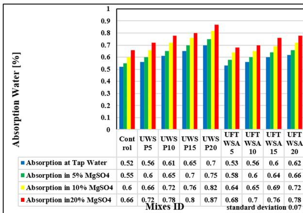
**Figure 13.** Absorption Water for Control, UWSP and UFTWSA for Tap Water and MgSO<sub>4</sub> Solution
