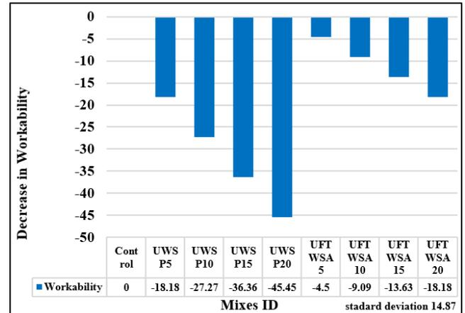
**Figure 7.** Reduction in workability of control, UWSP and UFTWSA mixes
