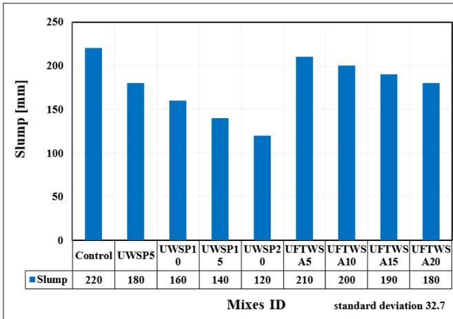
**Figure 5.** Slump flow for control, UWSP and UFTWSA mixes
