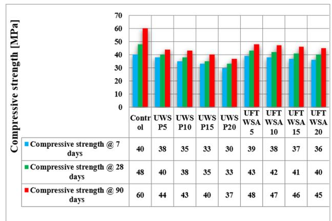
Figure 10. Compressive Strength for Control, UWSP and UFTWSA mixes
