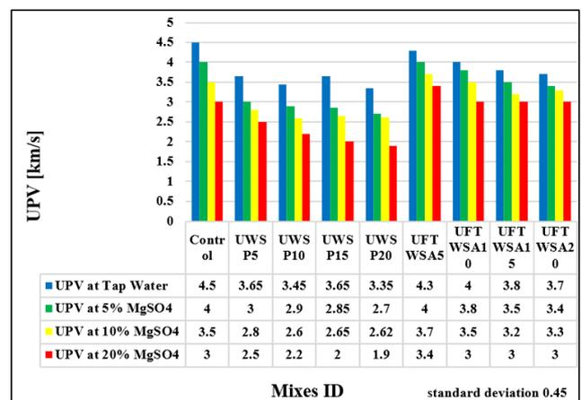
**Figure 15.** UPV of the specimens for control, UWSP and UFTWSA in tap water and MgSO<sub>4</sub> Solution
