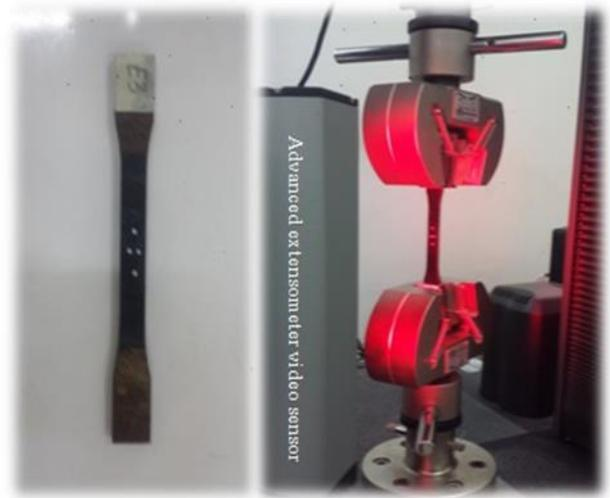
Figure 8. Video-tensile test
