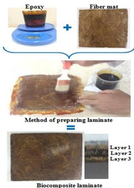
**Figure 5.** Method of preparing biocomposite laminate
