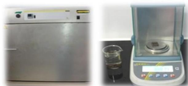
**Figure 6.** Water absorption test instrumentation
