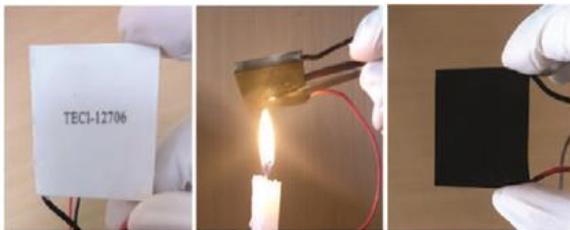
**Figure 1.** Candle-soot Method Coating system [22]
