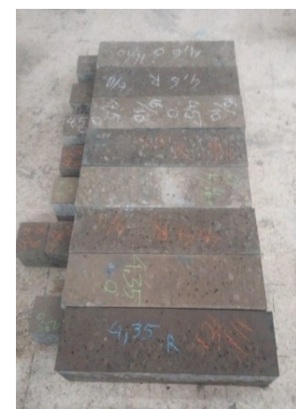
Figure 3. Specimens for flexural strength test (prism 150x150x600 mm)
