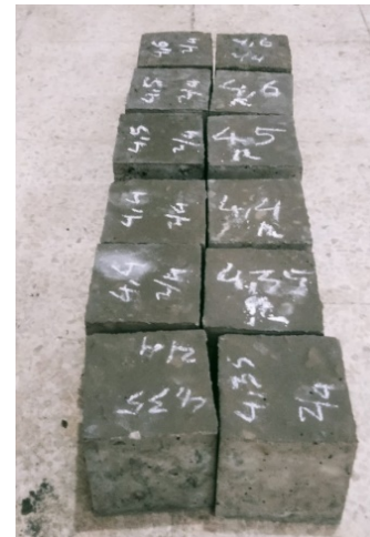
Figure 1. Specimens for compressive strength test (cube 100x100x100 mm)
