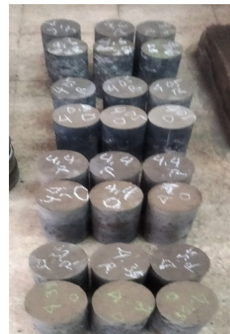
Figure 2. Specimens for tensile strength test and elastic modulus test (cylinders 150x300 mm)
