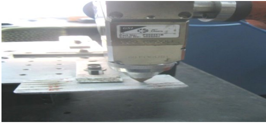
Figure 4. Experimentation of laser micro grooving during machining
