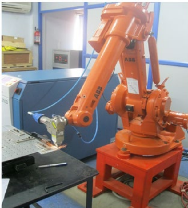
Figure 3. Experimental setup of Nd: YAG laser beam machine
