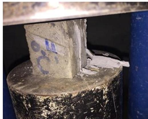
Figure 2. Compressive strength test for mortar cube
