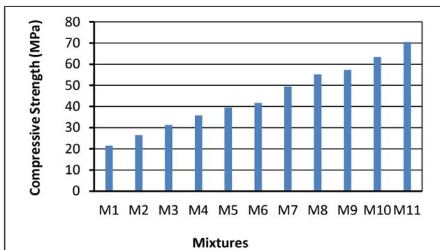
**Figure 3.** Compressive strength of geopolymer at 1 day with 24h curing duration
