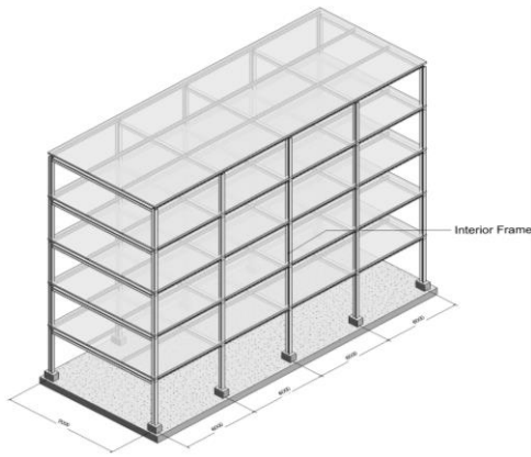
Figure 2. 3D view of multi-story moment resisting frame
