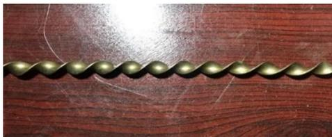
Figure 5. Twisted tape with T.R=2
