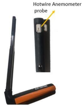
**Figure 2.** Testo hot wire anemometer probe
