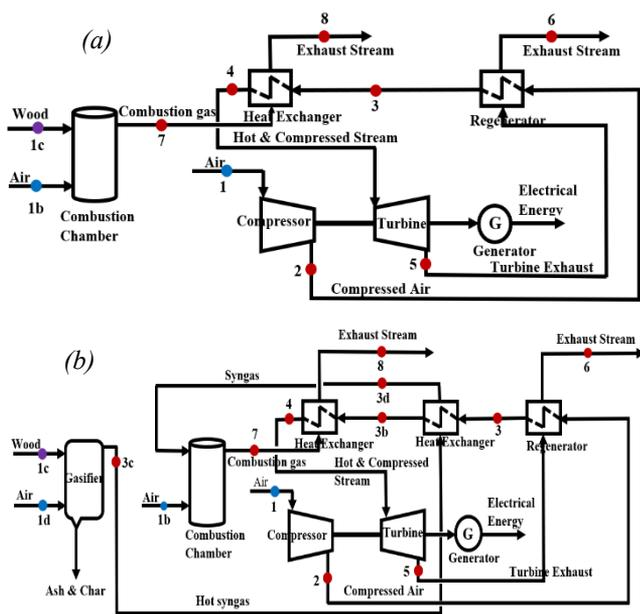
**Figure 1.** Schematic view of proposed plant for the conversion of wood to CHP through (a) WC-GT and (b) WG-GT configurations
