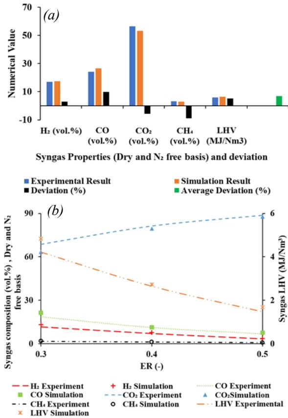
**Figure 2.** Difference between the results predicted through the developed model and the experimental outcomes during model calibration (a) and validation (b)
