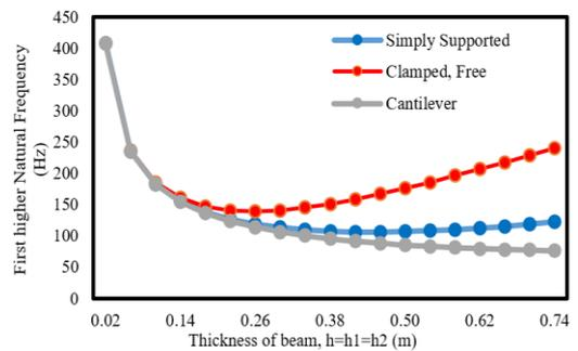
Figure 3. Higher natural frequencies versus thickness of double beam
