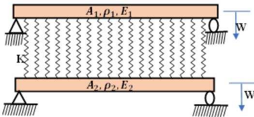
Figure 1. Double-beam with elastic connected layer
