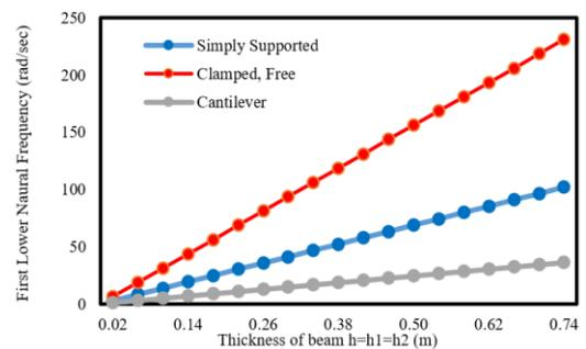
Figure 4. Lower frequencies versus thickness of beam
