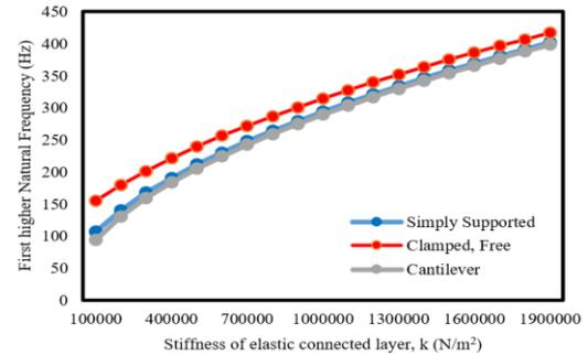
Figure 2. Higher natural frequencies versus stiffness of elastic layer
