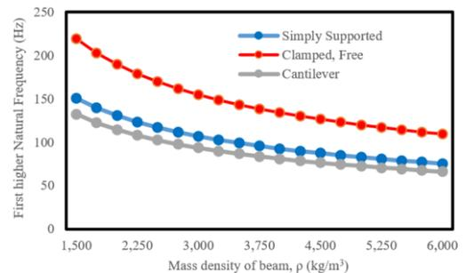
**Figure 7.** Higher natural frequencies versus mass density of double beam
