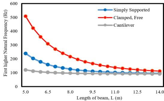
**Figure 9.** Higher natural frequencies versus length of double beam
