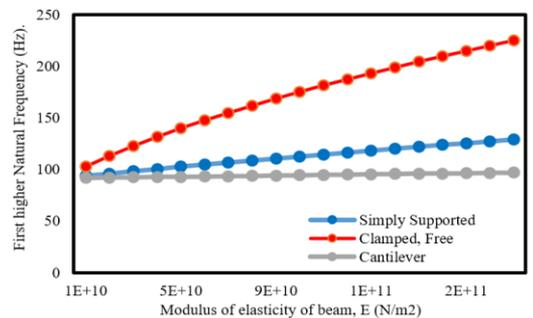
Figure 5. Higher natural frequencies versus modulus of elasticity of double beam
