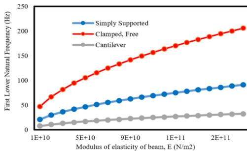
**Figure 6.** Lower natural frequencies versus modulus of elasticity of double beam
