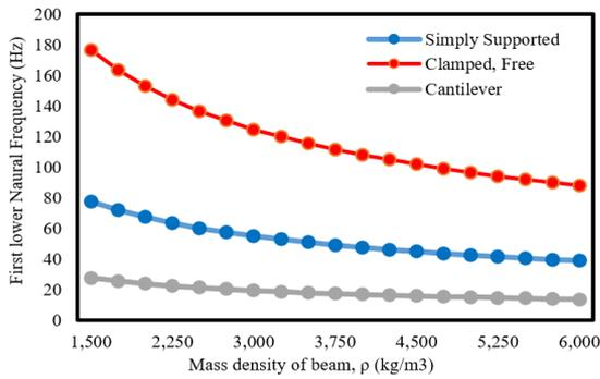
**Figure 8.** Lower natural frequencies versus mass density of double beam
