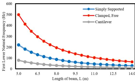
**Figure 10.** Lower natural frequencies versus length of double beam
