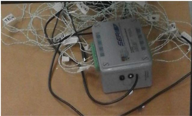
Figure 6. Data Logger ADAM-4019 for temperature data
