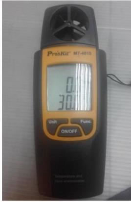
Figure 5. Anemometer for wind speed
