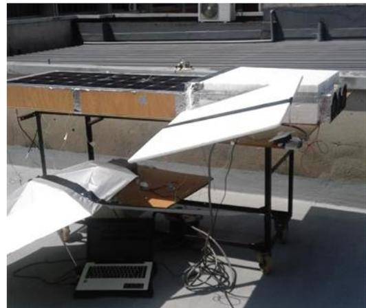
**Figure 3.** Outdoor investigation of photovoltaic thermal air collector
