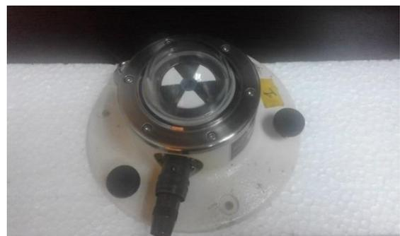
**Figure 4.** A pyranometer for sunlight radiation
