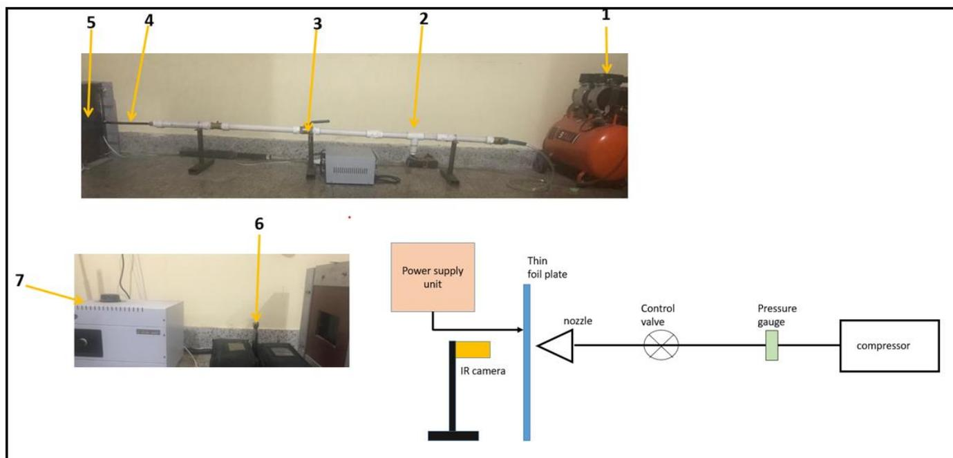
**Figure 1.** Actual setup and schematic diagram of experimental setup (1-Compressor; 2-Pressure Gauge; 3-control valve; 4-Nozzle; 5-Thin foil plate; 6-IR camera; 7- Power supply unit)
