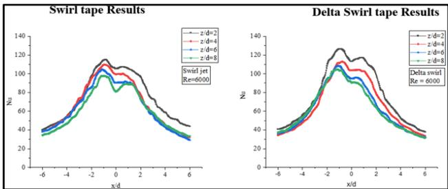
**Figure 15.** Centerline Nu distribution comparison for  $z/d=2$  to 8 and  $Re=6000$
