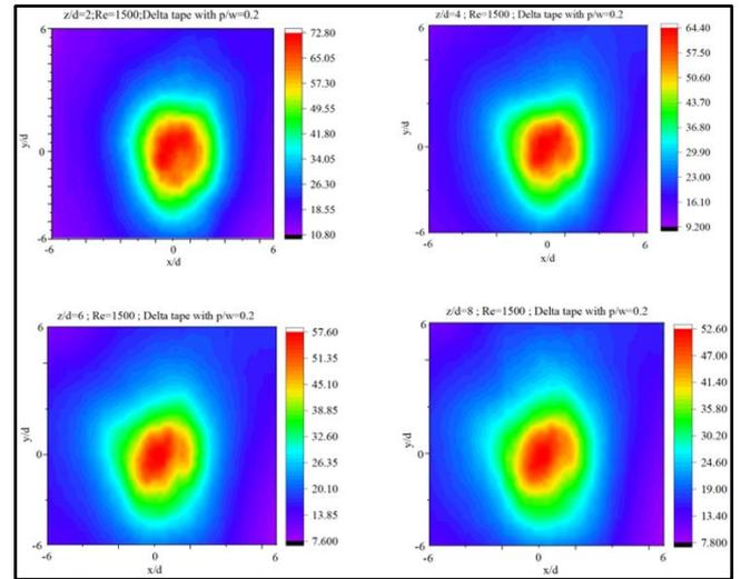
**Figure 17.** Contours of Nu distribution on target plate for  $z/d=2$  to 8 and  $Re=1500$
