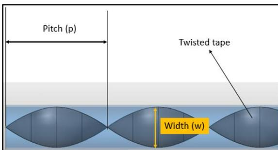
Figure 4. Twisted tape in the nozzle
