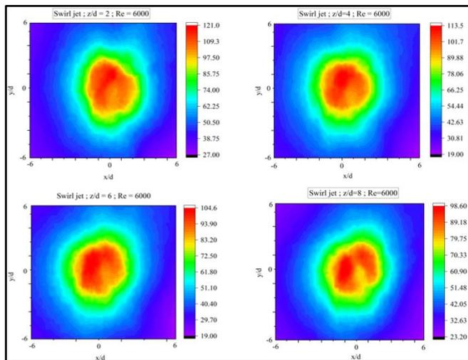
**Figure 10.** Contours of Nu distribution on target plate for  $z/d=2$  to 8 and  $Re=6000$
