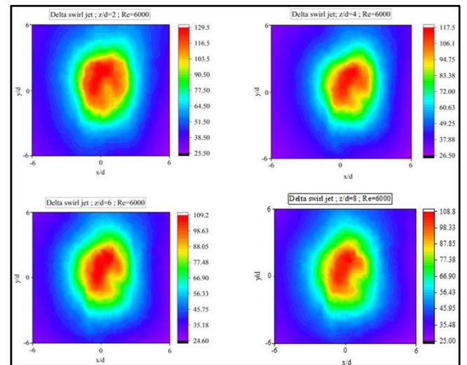
**Figure 19.** Contours of Nu distribution on target plate for  $z/d=2$  to 8 and  $Re=6000$
