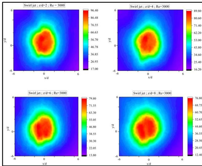
**Figure 9.** Contours of Nu distribution on target plate for  $z/d=2$  to 8 and  $Re=3000$
