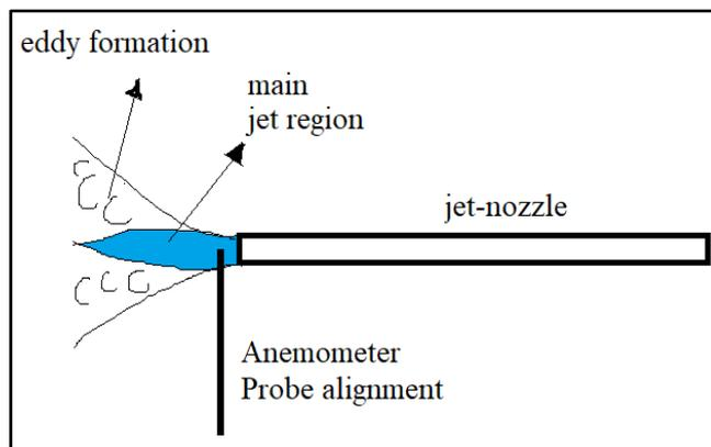
**Figure 3.** Probe position and alignment in jet flow
