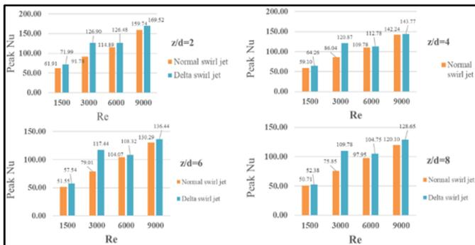
**Figure 21.** Peak Nu comparison for normal and delta tape case for  $z/d=2$  to 8 and  $Re=1500$  to 9000
