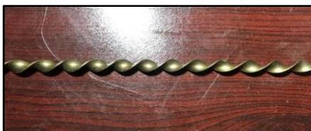
Figure 5. Twisted tape with T.R=2
