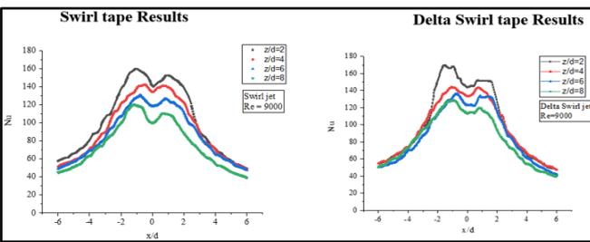
**Figure 16.** Centerline Nu distribution comparison for  $z/d=2$  to 8 and  $Re=9000$
