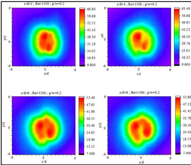
**Figure 8.** Contours of Nu distribution on target plate for  $z/d=2$  to 8 and  $Re=1500$
