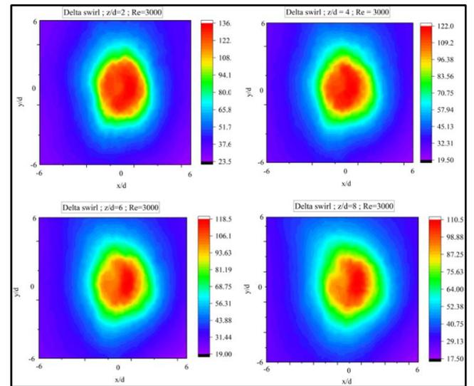
**Figure 18.** Contours of Nu distribution on target plate for  $z/d=2$  to 8 and  $Re=3000$
