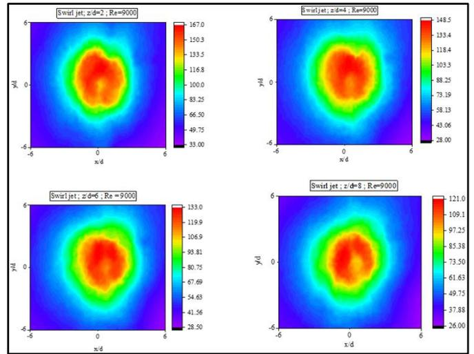
**Figure 11.** Contours of Nu distribution on target plate for  $z/d=2$  to 8 and  $Re=9000$
