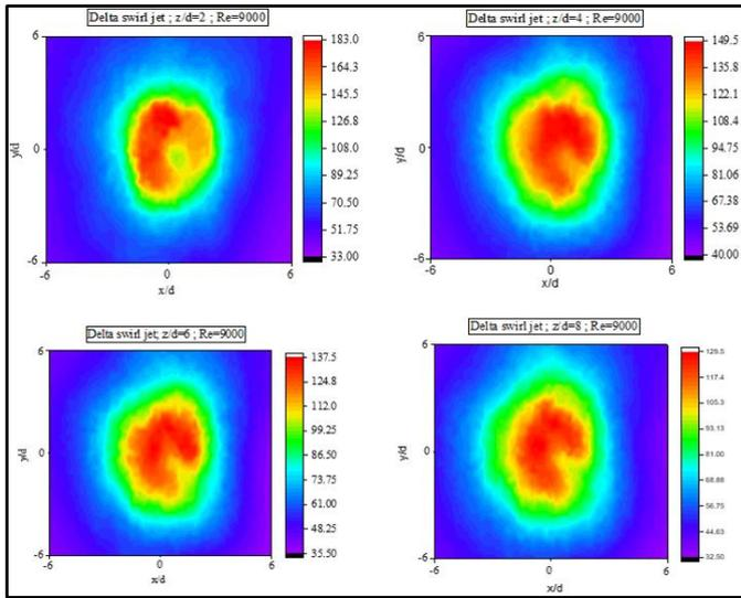
**Figure 20.** Contours of Nu distribution on target plate for  $z/d=2$  to 8 and  $Re=9000$
