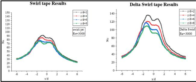
**Figure 14.** Centerline Nu distribution comparison for  $z/d=2$  to 8 and  $Re=3000$
