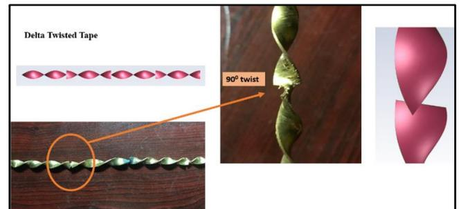
**Figure 12.** Delta Twisted tape
