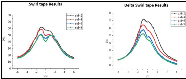
**Figure 13.** Centerline Nu distribution comparison for  $z/d=2$  to 8 and  $Re=1500$
