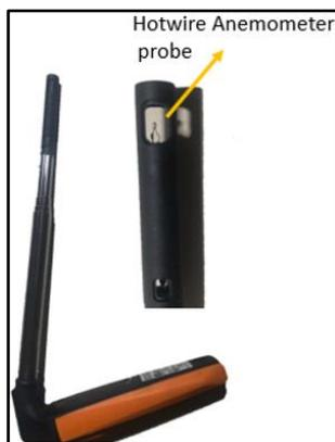
**Figure 2.** Testo hot wire anemometer probe
