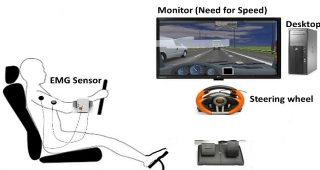
Figure 2. Experimental setup of the driving simulator
