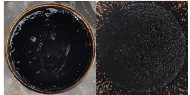
(a) RP-modified asphalt prepared by dry process (b) RP-modified asphalt prepared by wet process
