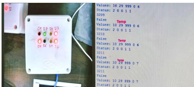
Figure 12. Temperature value 29 and turn off LEDS (D4 and D5)
