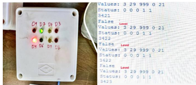
Figure 16. Level sensor value 3cm and turn off LEDS (D2&D3)
