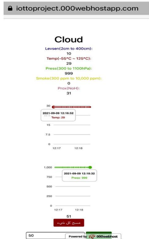
Figure 11. The values of the sensors with date in the cloud
