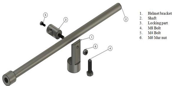
Figure 4. BC3 boccia helmet stick assembly
