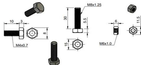
Figure 6. Bearing (Nut and Bolt)
