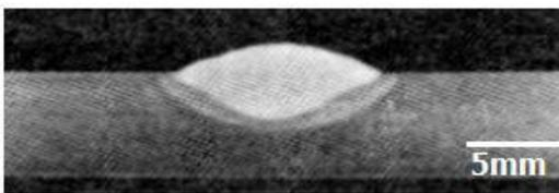
Figure 7b. Image macroscopic the effect of minimum welding speed Without nanoparticles
