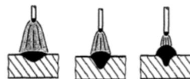
**Figure 6.** Change voltage in wire feed speed constant welding the weld penetration [10, 11]
