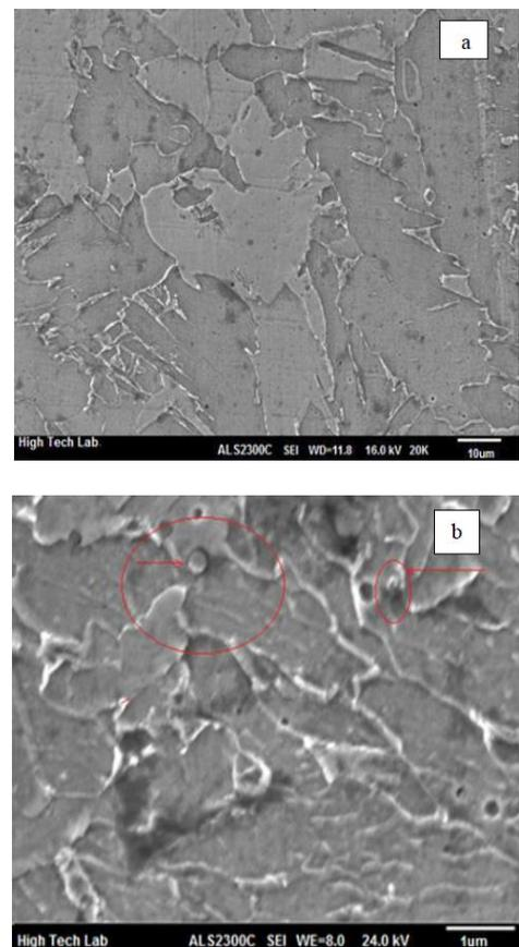
**Figure 11. a.** The weld metal microstructure Without nanoparticles (No.22)-**11b.** The weld metal microstructure with nanoparticles (No.32)
