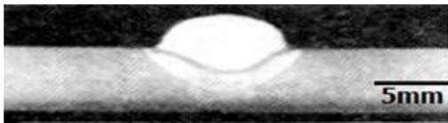
Figure 7a. Image macroscopic the effect of maximum welding speed Without nanoparticles (sample No. 23)
