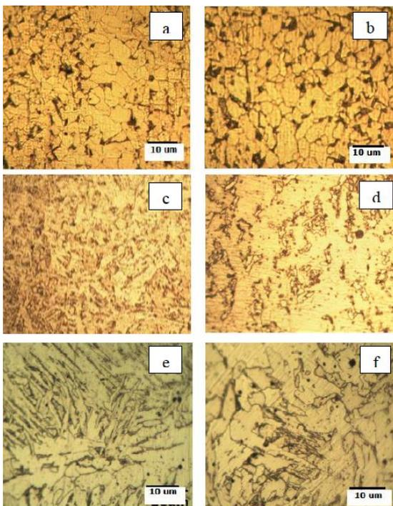
**Figure 10.** Optical microscope images of different welding regions. a,b: Metallographic image of base metal: (a :Sample 32), (b: Sample 22). c,d : HAZ metallographic image: (c: Sample 32), (d: Sample 22). e,f: Metallographic image of weld metal: (e: Sample 32), (f: Sample 22)
