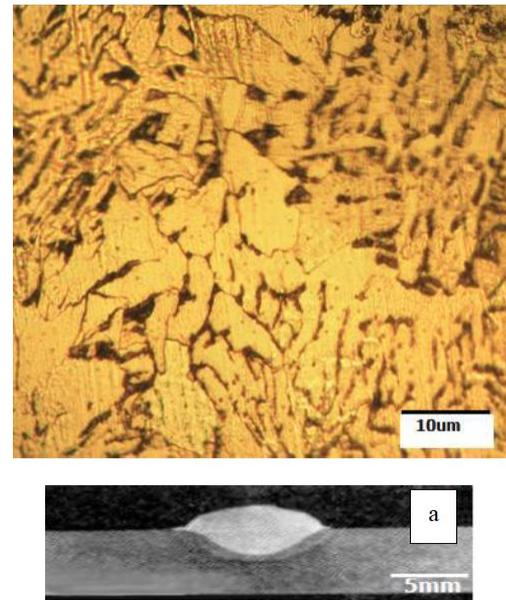
**Figure 4.** Microscope image of the microstructure of weld metal, a macroscopic image of the flow rate effect (sample No.18)
