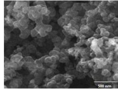
Figure 1. SEM of ZrO<sub>2</sub> nano-particles
