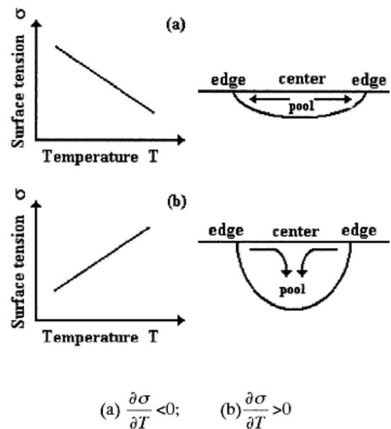
Figure 8. Marangoni convection mode by surface tension gradient in welding pool (a)  $\partial\sigma/\partial T < 0$ ; (b)  $\partial\sigma/\partial T > 0$  [18, 19]
