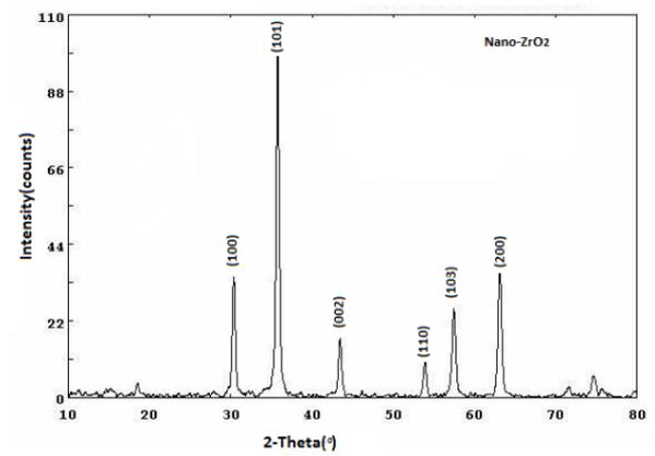
Figure 2. XRD of ZrO<sub>2</sub> nano-particles
