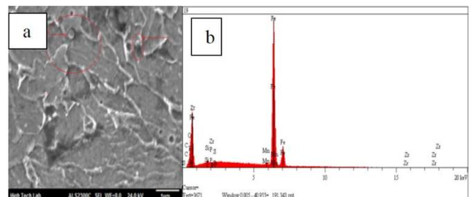
**Figure 12.** (a) SEM 1micrograph showing the nucleation of acicular ferrite laths on inclusion in weld A2, (b) EDS analysis on the inclusion in (a)
