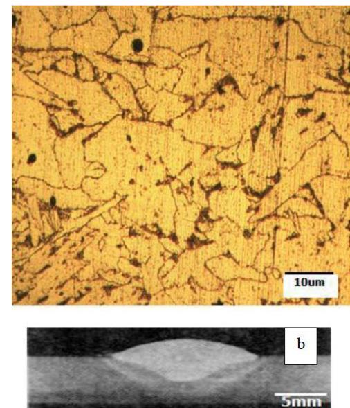
**Figure 5.** Microscope image of the microstructure of weld metal, a macroscopic image of the flow rate effect (sample No.19)
