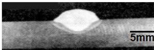
Figure 7c. Image macroscopic the effect of maximum welding speed the thickness of the layer 0.5mm nanoparticles (sample No. 4)
