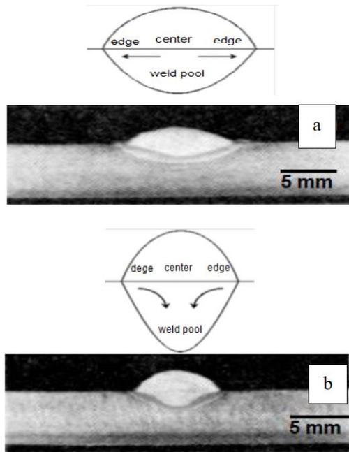
**Figure 9.** Image macroscopic the effects of nanoparticles on the geometry and weld penetration (sample No. 22&32)
