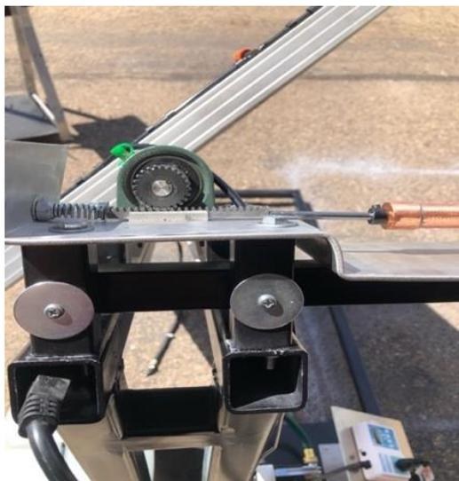
Figure 3. Rack and pinion gear system
