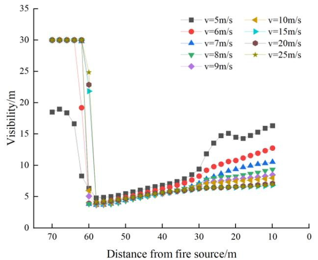
Figure 7. Distribution of visibility at a height of 2m on the right side of the fire source
