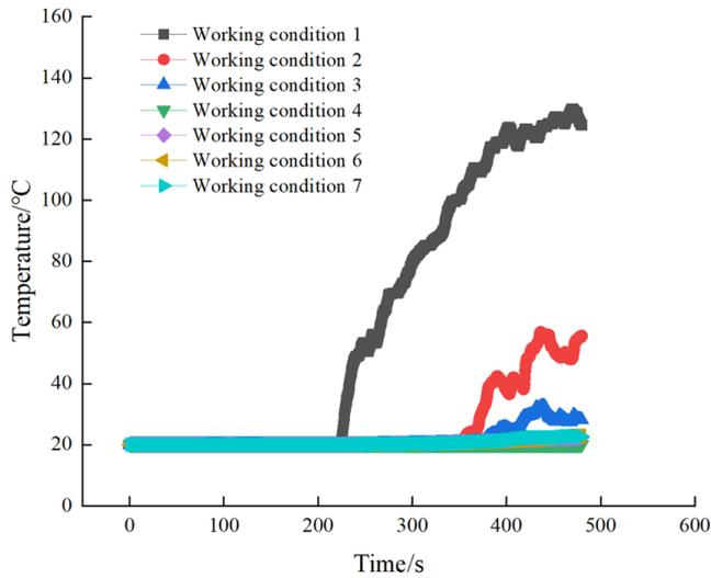
**Figure 5.** Temperature distribution at the ceiling of the tunnel
