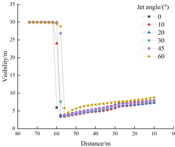
Figure 10. Distribution of visibility at different jet angles
