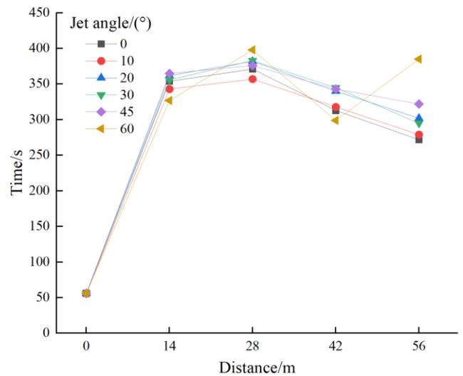
Figure 12. Distribution of the time it takes for the temperature at each measuring point to reach the critical value
