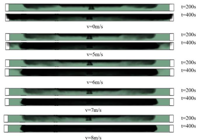
Figure 3. Smoke spread at different jet velocities
