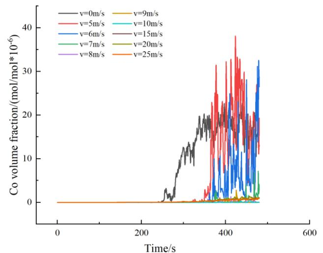
Figure 8. Distribution of CO concentration at 2m height in the escape area
