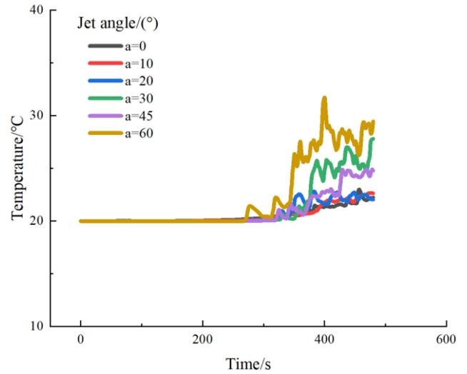
Figure 11. Distribution of temperature in the escape area at different jet angles
