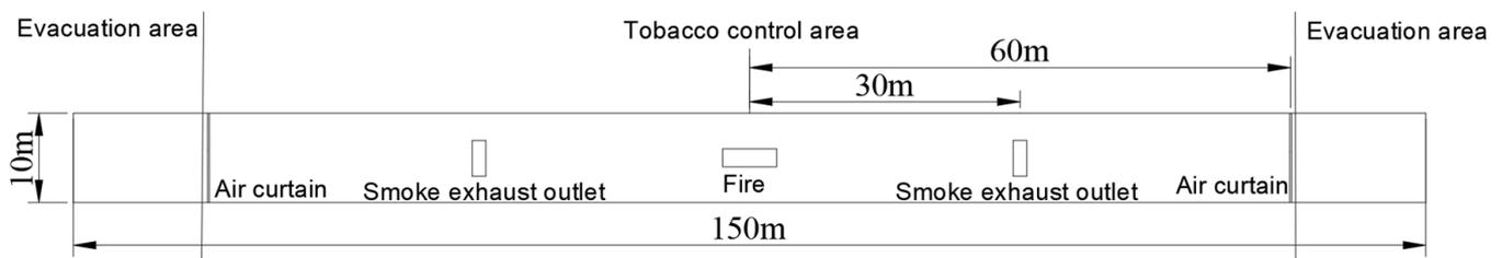
Figure 1. Model of the tunnel
