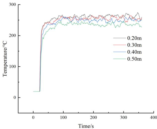
Figure 2. Distribution of ceiling temperature under different grid sizes
