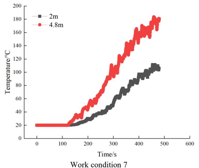
**Figure 6.** Temperature distribution at different heights
